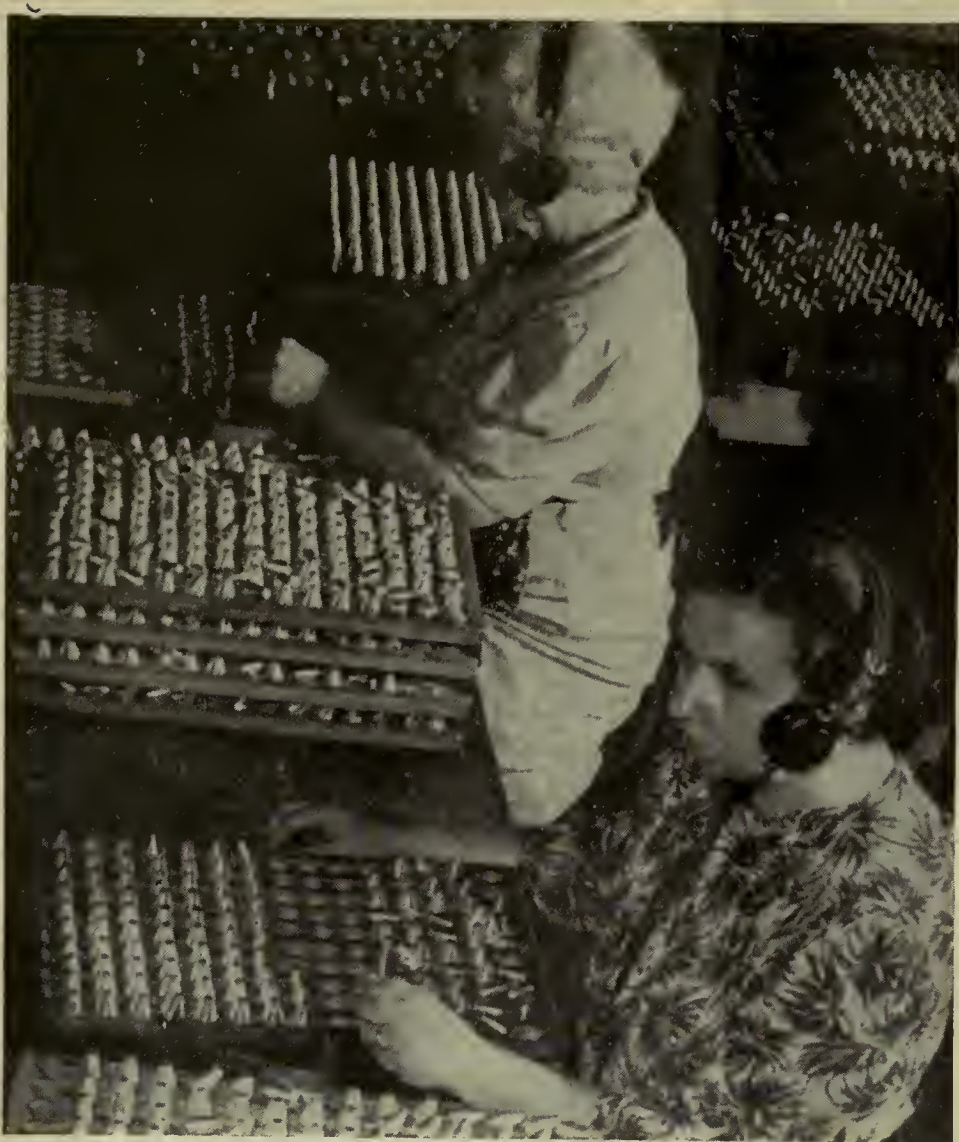
Inspectors at Stewart-Warner listen for flaws in shell fuze heads
